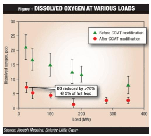
When operating at full load, DO levels at Little Gypsy were acceptable. When operating at lower load, DO was considerably higher (Figure 1). Being a peaking plant, Little Gypsy ran at an idle power of 20 to 40 MW half the time. At this low operating level, DO reached high levels that were unacceptable to plant owner, Entergy Corp., and proved problematic for the plant (Figure 2).
