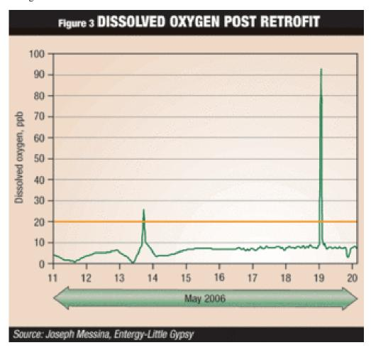
After the retrofit was completed and the unit was returned to operation last spring, the results were immediate and dramatic (Figure 3). At 22 MW, DO decreased from 22 parts per billion (ppb) to 7 ppb and at 180 MW DO decreased from 13 ppb to 2 ppb. The guaranteed projection level was 10 ppb. Intek's unique understanding of condenser dynamics was a key to the program's success.
