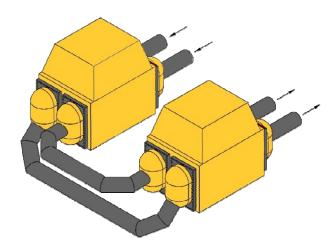
In 2007 Intek was presented with an opportunity to study an underperforming Ingersoll Rand condenser, and plan a program for increasing performance via engineered retrofit. The primary objectives for the condenser study were to find a means to mitigate ongoing load limiting conditions in the summer time due to high condenser pressure and to improve chronic poor condenser performance, which had continued despite maintaining excellent tube cleanliness with an online ball cleaning system.
